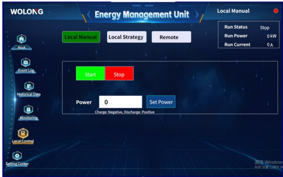
Figure 8-6 Local Control Interface
