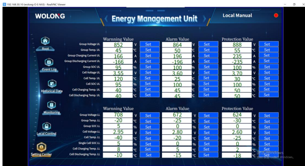
Figure 8-9 Settings Center (Protection settings)
